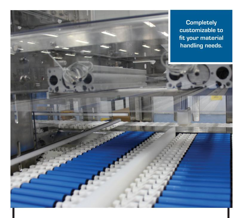
Adaptable to many different applications, the Pusher Station is an ideal solution for sorting specific product from the main conveyor flow. Its rugged construction is suitable for heavy products and ideal for product sorting, palletizing and product reject systems.
