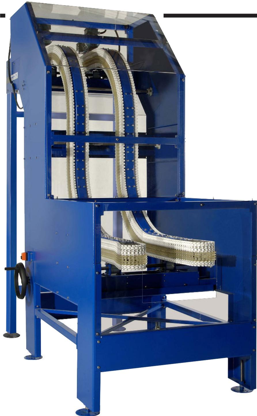
You can see the wedge in motion, but you probably won't hear it. The almost-silent unit is designed with all-mechanical movement, gripping products on their sides and sending them on their way. Don't have much floor space? It's not a concern for the compact Wedge units.
