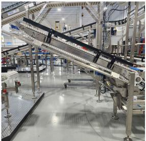
When personnel or equipment require access to the interior of a an area of your facility that is blocked by a conveyor, a lift gate can be the solution. Our lift gate is a counter-weighted or spring-loaded conveyor section, hinged to allow it to be raised and lowered as needed. The Lift Gate is designed to safely remain in the "up" position after being raised, until it is intentionally lowered. The Gate's conveyor section can be slave-driven from the preceding conveyor, if desired.
