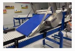
The Span Tech Vertical Switch Conveyor is an innovative solution designed to handle complex, multi-level product sorting and distribution with ease and precision. Actuated by pneumatics or manually switched, Vertical Switch Conveyors Allow for the merging of non-rigid products. It can also be used as a reject.
