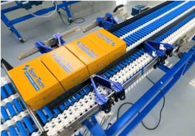
Tube Top chain was created so that more products could be accumulated than what was possible on plain chains. Tube Top Chain can incline or decline 2°
