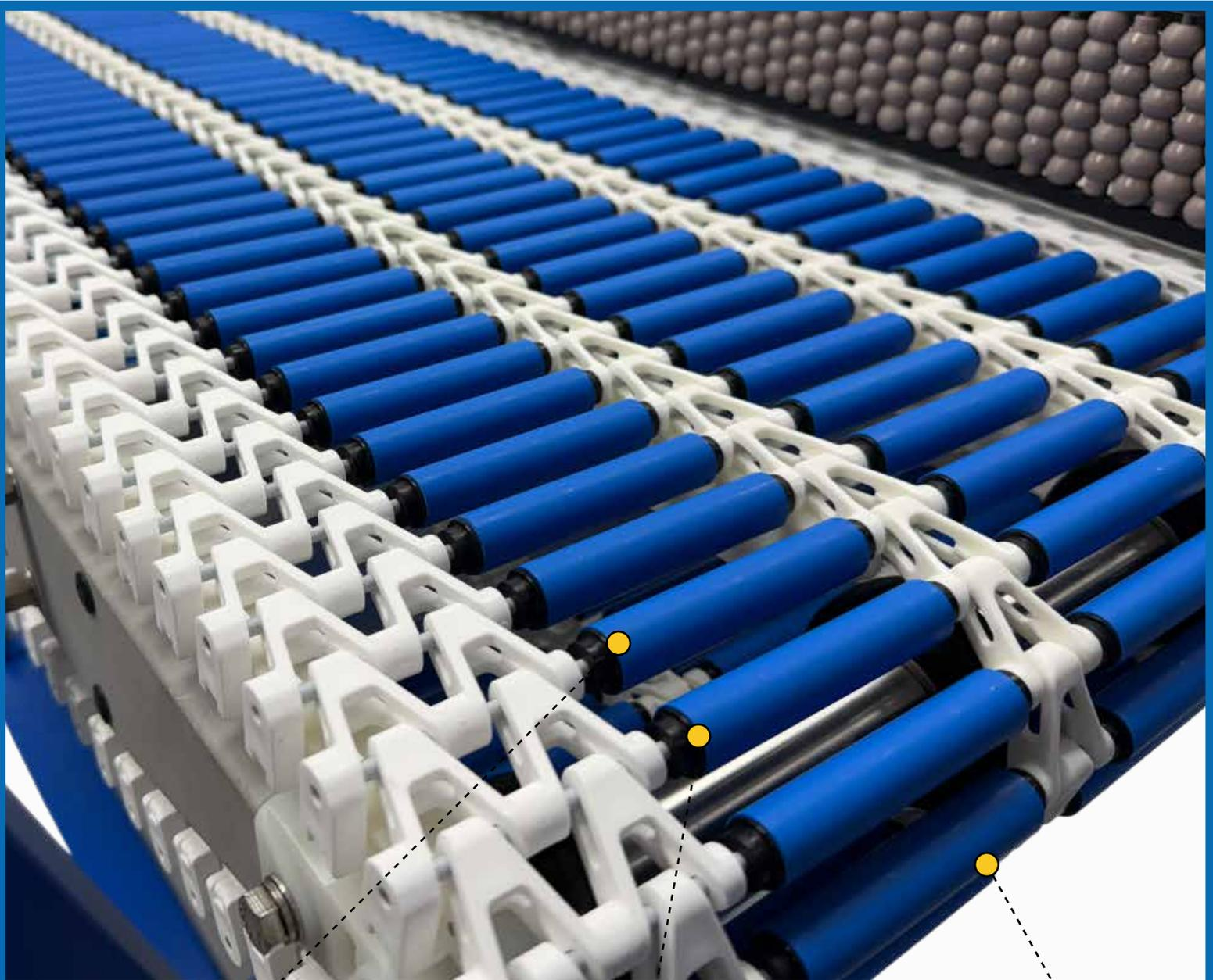
Tube Top Rollers reduce back pressure allowing products to accumulate easily without damage.
