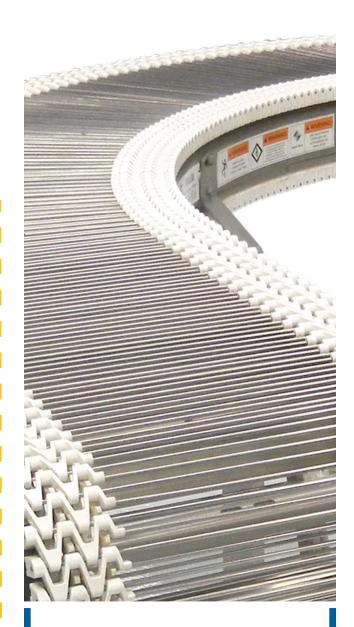
The smarter way to move and cool food products. The J-Trax system adds efficiency to the food and beverage industry which comes with its own unique set of challenges. J-Trax is easy to install and ideal for any family of food products. The functional design and no wire-to-wire friction allows for a chain type with greater durability and endless applications.
