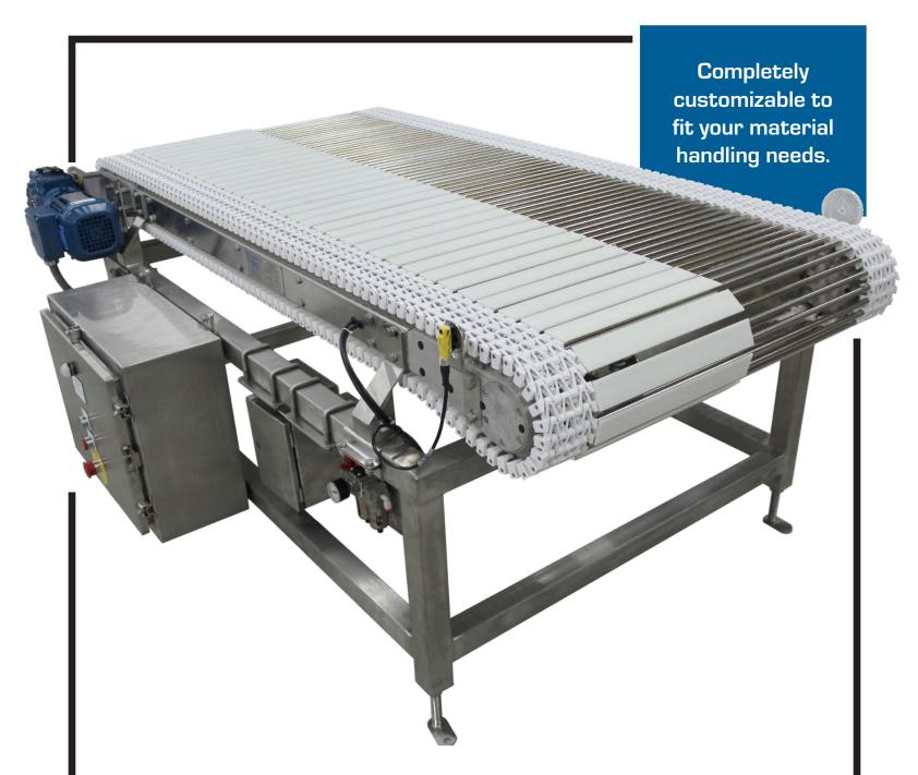
Need to split product flow quickly and reliably? And at speeds that can't be overlooked? We currently have high-speed switches splitting product flow at up to 400 fpm. Products are transferred along by a series of carriers which are supported by guide rods. Everything is powered by a pair of MonoSpan conveyor chains. 1:2, 2:3, etc. or can be programmed to divert a product whenever you need it. Contact us for options.
