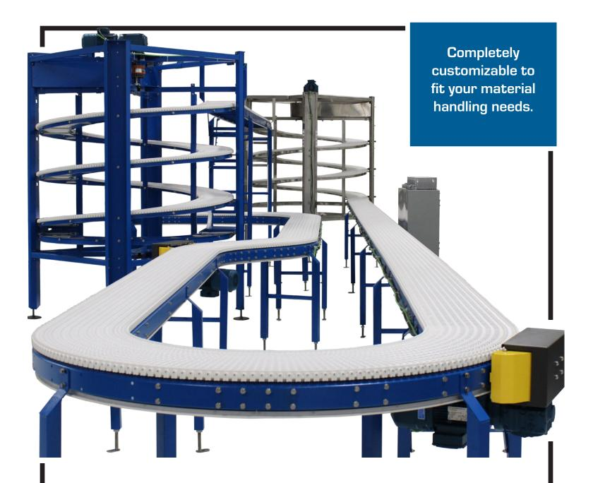
A cost effective solution for changing elevations, the Outrunner Spiral Elevator conveyor gives you the capacity to move several product types without taking up valuable floor space. For an elevation change with a minimal footprint spiral elevators are ideal. The cost-effective, compact units are not only strong, but gentle as well. No pressure is applied to the product, so even delicate items can pass through it without damage.
