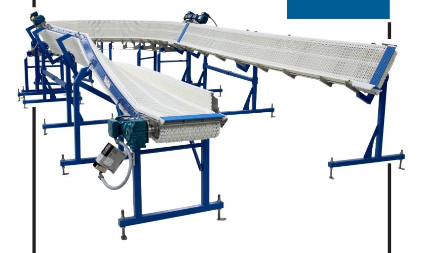
Our Twist Conveyors can be used for easy and foolproof product orientation or to precisely align items as required for downstream processes. Depending on the specific need, products can be reoriented by any angle up to a full 90 degrees. If a conveyor is twisted along the axis of the side frame, the product will maintain the same elevation. If the twist is along the conveyors center line, a natural decline of the product will occur.
