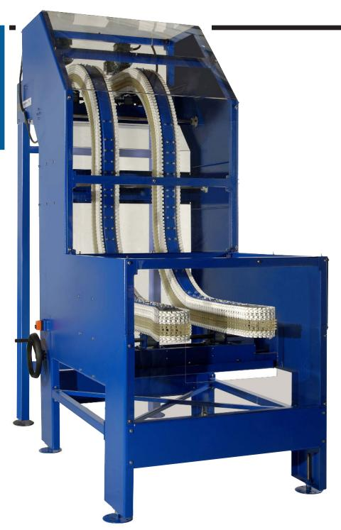
You can see the wedge in motion, but you probably wont hear it. The almost-silent unit is designed with all-mechanical movement, gripping products on their sides and sending them on their way. Don't have much floor space? It's not a concern for the compact Wedge units.
