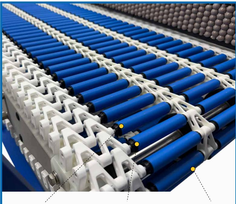
Tube Top Rollers reduce back pressure allowing products to accumulate easily without damage. The tubes rotate freely on the stainless steel rods, acting as a roller allowing the chain to easily run under a stationary product without damaging it.
